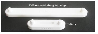
to each flange. C-Bars are longer and are only used on 5 ft or larger looms. They go from the center holes in each module to the center hole of the adjacent module on standard gauge looms and from one hole next to a flange, over a module into the nearest hole of the next module in fine gauge looms.
